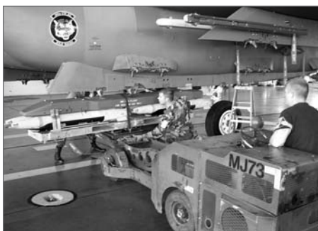
Mountain Home AFB, Idaho — A load crew airman uses a jammer to attach a pair of GBU-39 bombs to an F-15E Strike Eagle.
